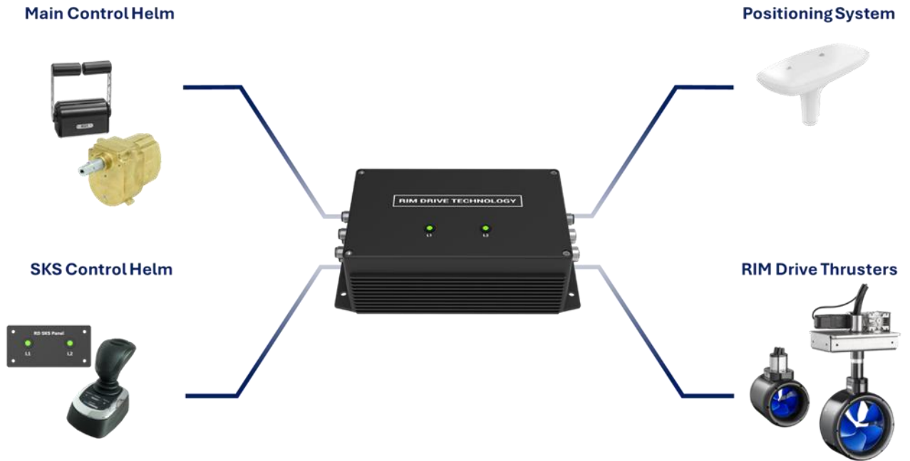
Figure 1: System Block Diagram
