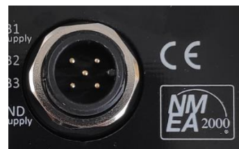
Figure 4: M12 N2K connector on SMARTSHUNT
