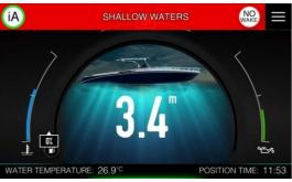
When IAssist screen is displayed, green icon with iA label will be drawn in top left corner of the screen. Press it to dismiss IAssist screen.
