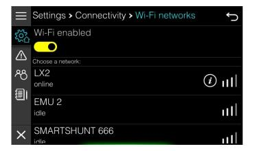
If you are already connected a round icon with letter i will be shown next to signal strength. Press it, to get information about IP address assigned to the device.
