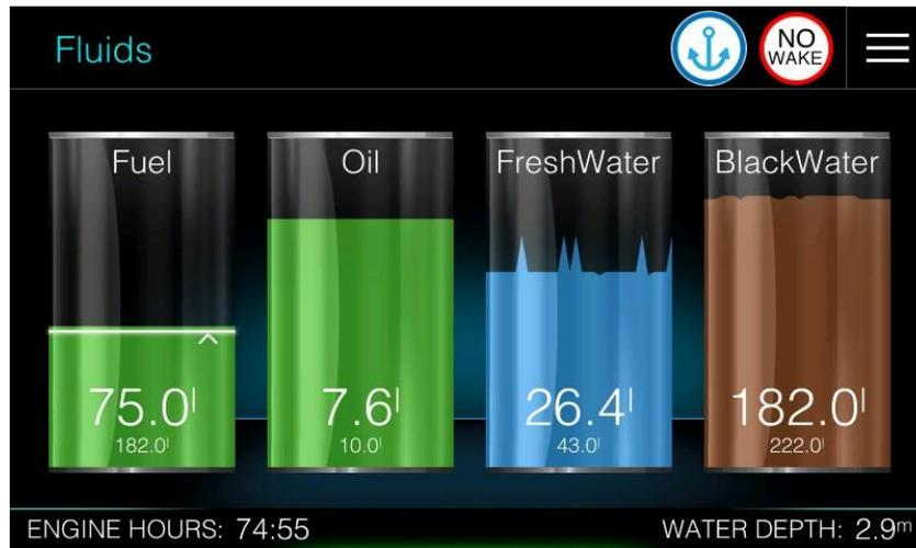
Fuel tank is a bit special. When measured fuel and calculated fuel data are available, measured data is presented as any other fluid level, with a time series graph as a level. Calculated data is drawn with a white line and a pointer on the right side.
