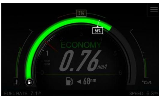
When a fluid level sensor is connected to network, green arc will display averaged measured quantity and white pointer will show calculated fuel. If only calculated fuel is available, white pointer will always be at the end of arc. White pointer is not drawn, if only measured fuel is available.
