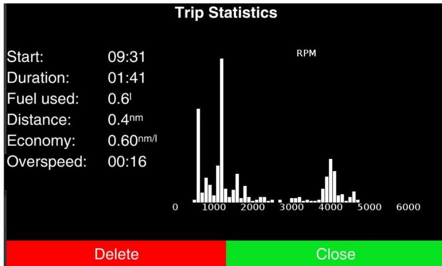
Start of current trip and its duration. Duration is taking into account only time, when engine was running. Fuel used during trip. Distance covered. Fuel Economy, which is calculated based on distance covered and fuel used during duration of this distance being done. Overspeed time is time, when vessel was travelling about set high speed and above no wakezone speed. Histogram on the right displays which RPM were used most of the time during the trip.
