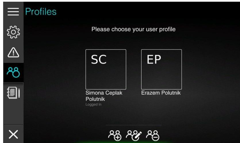
A list of profile is shown in boxes with initials. A full name of profile is printed below the box. The profile, which is currently being used is identified with Logged in label below the name.
