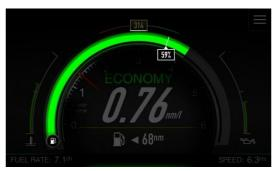
When a fluid level sensor is connected to network, green arc will display averaged measured quantity and white pointer will show calculated fuel.
