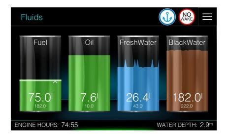
Fuel tank is a bit special. When measured fuel and calculated fuel data are available, measureddata is presented as any other fluid level, with a times series graph as a level. Calculated datais drawn with a white line and a pointer on the right side.
