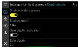
On your device you can set two different depths. First one is call safe depth and the other one is called shallow waters. This allows you to setup two stage depth warnings.
