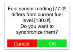
Calculated fuel and measured fuel are both shown od dashboard screens, fluid screen and chart screen. User can also set a floating box with both values.
