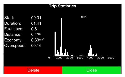
Start of current trip and its duration. Duration is taking into account only time, when engine was running. Fuel used during trip. Distance covered. Fuel Economy, which is calculated basedon distance covered and fuel used during duration of this distance being done. Overspeed time is time, when vessel was travelling about set high speed and above no wakezone speed. Histogram on the right displays which RPM where used most of the time during the trip.
