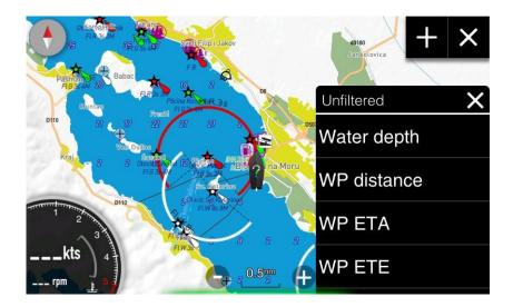
Select your desired parameter from the list. By default all possibilities are shown, if you would like to get a filtered view, press on top row (Unfiltered) and select a filter from a list of choices (unfiltered, engine, fuel, trip, vessel status, environment, route, time and battery).
