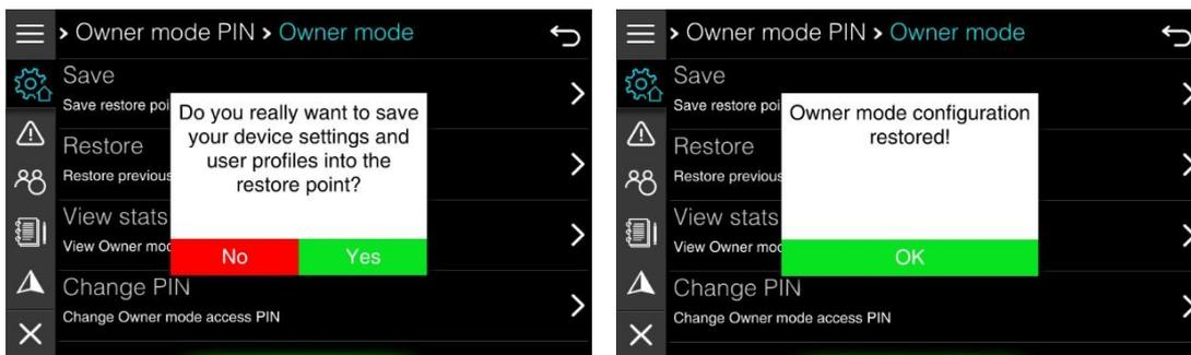
Only one restore point is saved to the SD card. If you have previously saved a restore point to SD card, it will be overwritten with new restore point.
