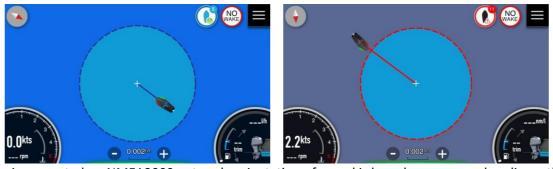
If compass is presented on NMEA2000 network, orientation of vessel is based on compass heading, otherwise vessel is always pointing towards anchor position.
