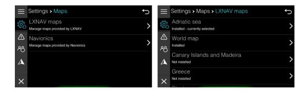
A list of all available maps data is shown together with indication, if it is installed or not. Selected item you would to manage. A new screen will open as shown on picture below.
