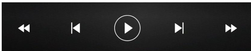
When playing music from USB or BT most left and most right button will fast forward or backward current song. Inner two forward and backward buttons will move to next/ previous song. Press middle button to toggle play or pause. When playing radio, middle button is not used. Inner forward and backward button are used for channel scan and will stop at nearest radio station. Outer buttons are used for frequency scan.
