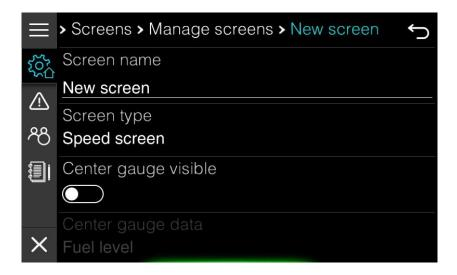
It is possible to select among following dashboard templates: speed screen, position, fueleconomy screen, depth screen, fluids screen, battery screen, trim screen and rudder screen. You can also select map screen template or audio screen template. Customization options vary depending on screen type. More details about dashboard screenoptions were given in chapter 5.
