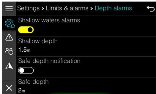
On your device you can set two different depths. First one is called safe depth and the other one is called shallow waters. This allows you to setup two stage depth warnings.
