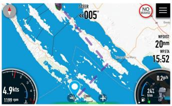
Dashed polyline from your vessel position via intermediate points towards final destination willbe displayed. Once route is calculated, it will be displayed in green colour with all parameters recalculated.
