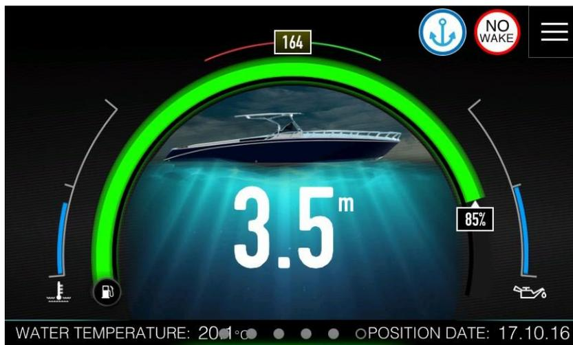
The dashboard screen is also used for IAssist function. The idea of dashboard screen is to show to the operator the right information at the right time. A smart logic is built-in device to choose right screen for a given situation. There is no need for the operator to search for requested parameter. A single most important value is shown on the centre of the screen
