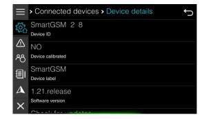
Select a device to get more details about it. At the bottom of the device details, there is an option to reset configuration for this device. This will delete all configurations previously donefor this device and device will behave as being seen for the first time. Externally connected devices manufactured by RIM DRIVE TECHNOLOGY will have an option to upgrade software. Select item Check for update to update it and follow instructions given.
