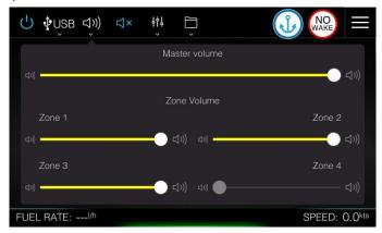
Number of zones may vary from audio device to audio device. Press mute icon to mute audio instantly. When radio is muted, icon will be in blue colour. Repressing it will restore volume level to previously set level.
