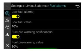
For fuel you have also two stage warning system. Fuel pre-warning value will generate informational warning (white). Low fuel value will generate important warning.
