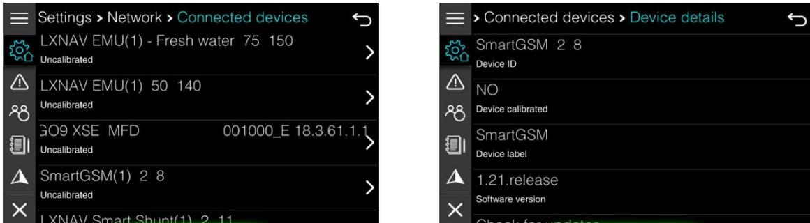
Select a device to get more details about it. At the bottom of the device details, there is an option to reset configuration for this device. This will delete all configurations previously done for this device and device will behave as being seen for the first time. Externally connected devices manufactured by RIM DRIVE TECHNOLOGY will have an option to upgrade software. Select item Check for update to update it and follow instructions given.
