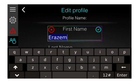
Once you have finished entering text, press red X icon to cancel editing and exit without savingchanges. Press ENTER button on keyboard or blue checkmark to confirm changes and exit editing mode. Press UP arrow to switch to upper case letters. If you would like to do CAPS LOCK double, click UP arrow.
